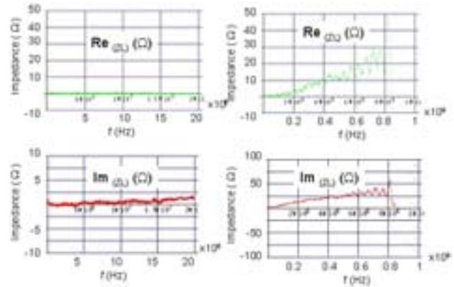
Figure 3: Longitudinal impedance measured by the coaxial wire method. The upper figures are real part of impedance and the bottom figures are ones of imaginary part. The left figures are the longitudinal impedance in the range of less than 20 MHz, and right figures are ones in the range of 1 GHz.
