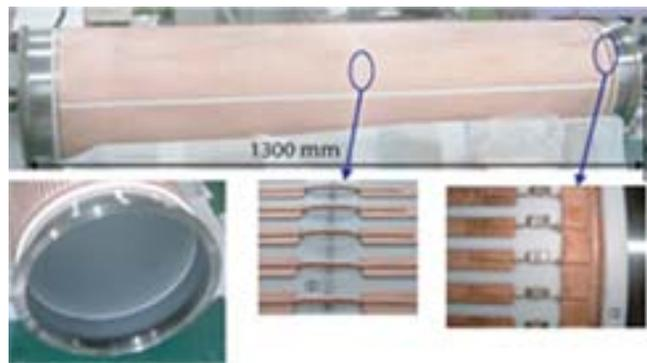
Figure 1: Picture of the alumina ceramics vacuum duct for quadrupole magnet. (1) TiN coating : Thickness is about 15 nm. (2) Duct joint : Each duct is jointed with metallizing and brazing, and any Cu stripes are bridged over the brazing joint in order to be electrically insulated from each other. (3) Capacitor : Capacitors are welded between each Cu stripes and titanium flange. The capacity is 330 nF.
