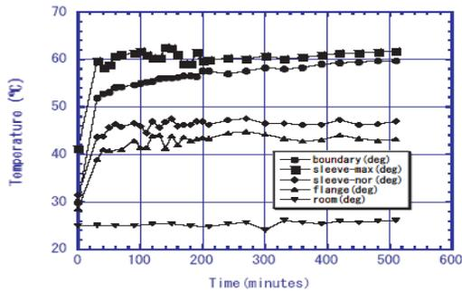
Figure 2: Temperature of the titanium flange and sleeve under normal operation of dipole magnet. The dipole magnet operation conditions were 25 Hz repetition and magnetic field changing from 0.17 T to 1.1 T.
