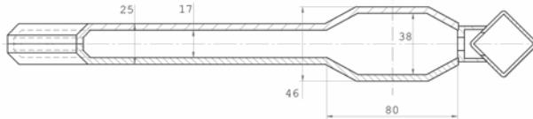
Figure 4: Cross section of steel chamber in new octant. The NEG pumping channel is located on the right side.
