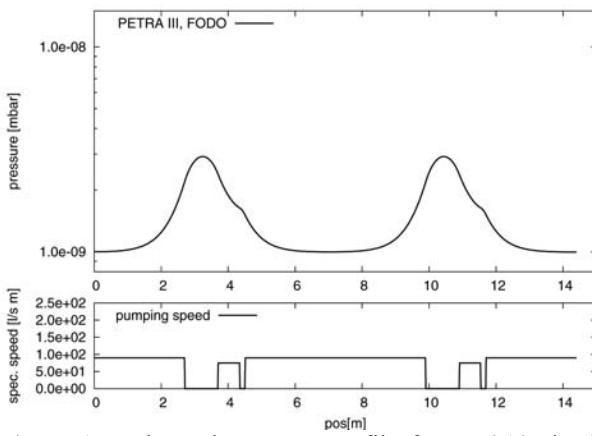
Figure 1: Estimated pressure profile for  $\eta=6 \cdot 10^{-6}$  in the standard arc.
