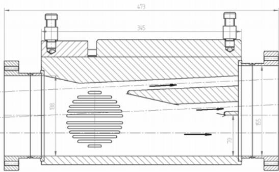
Figure 5: Copper absorber for dipole radiation with three openings for two undulator beams and the circulating particle beam.
