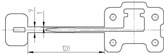
Figure 6: Cross section of the proposed wiggler chamber. The NEG pumping channel is visible on the right side.
