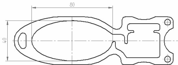
Figure 2: Cross section of the dipole chamber. Synchrotron radiation is absorbed on the left side. The NEG strip is located in the right handed side channel.
