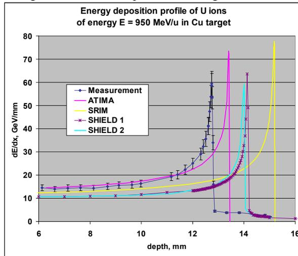
Figure 8: Comparison of the measured and calculated energy deposition profiles dE/dx for the case of 950 MeV/u U ions in Cu target.
