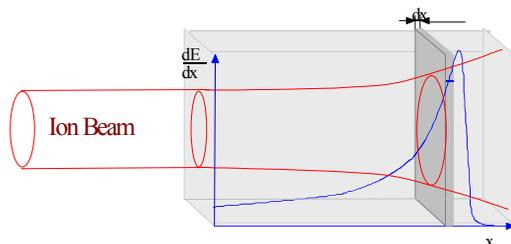
Figure 1: The scheme of the "thick target" method
