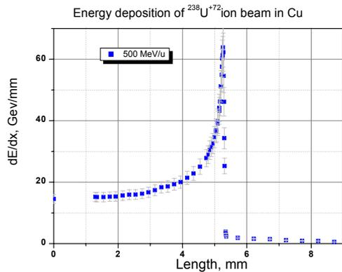
Figure 4: Energy deposition of  $^{238}\text{U}^{+72}$  ion beam with 500 MeV/u energy in Cu
