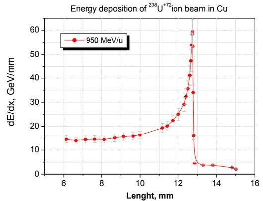
Figure 5: Energy deposition of  $^{238}\text{U}^{+72}$  ion beam with 950 MeV/u energy in Cu
