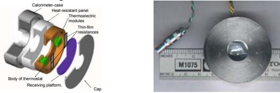
Figure 3: Schematic view and photo of the calorimeter
