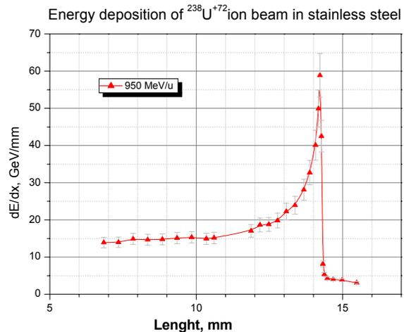
Figure 7: Energy deposition of  $^{238}\text{U}^{+72}$  ion beam with 950 MeV/u energy in stainless steel
