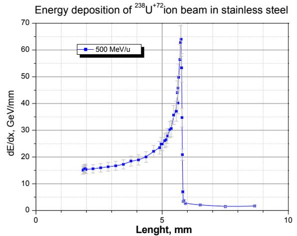
Figure 6: Energy deposition of  $^{238}\text{U}^{+72}$  ion beam with 500 MeV/u energy in stainless steel
