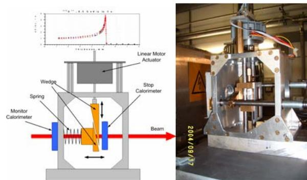
Figure 2: Scheme and photo of the manipulator
