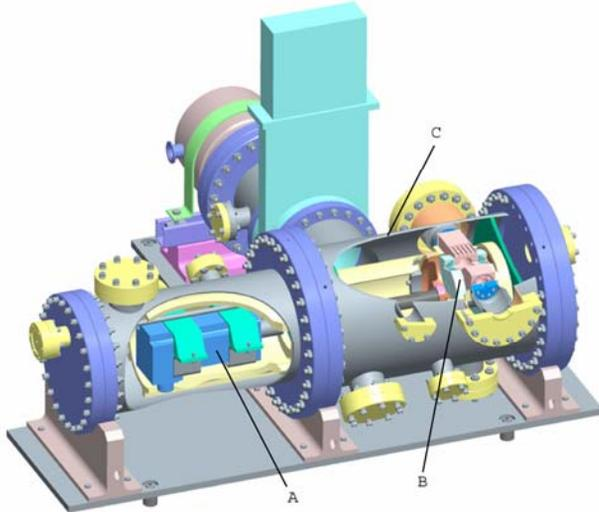
Figure 5: Details of the rotating aperture assembly including the motor (A), the cross flow tube and rotors (B), and the vacuum vessel (C). The overall length of the system shown is 1.2 m.
