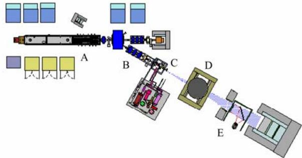
Figure 1: Drawing of a 7-MeV deuteron linac (A) coupled to the high energy beam transport (B). The beam makes neutrons in the gas cell (C), which then pass through the object (D) and produce an image on a plastic scintillator that is transported through an optics system to a CCD camera (E).
