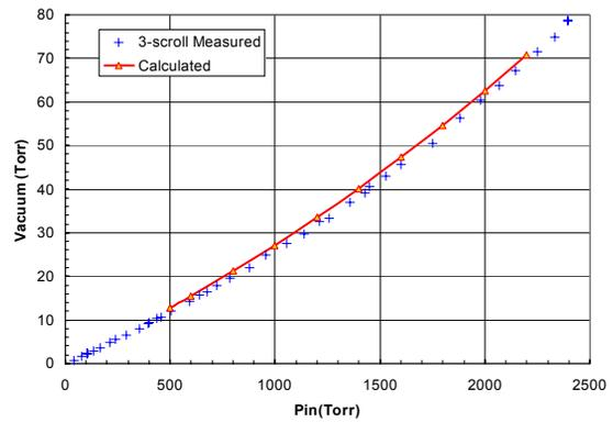
Figure 6: Plot showing the dynamic leakage of gas through the rotating aperture system compared to modeling (red line) Data is for helium gas and apertures set for a 2% duty factor beam.
