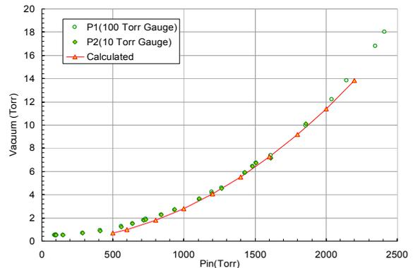
Figure 7: Static leakage results with the holes not aligned indicate the extent of leakage through the rotor-cross-flow gap compared to model (red line).
