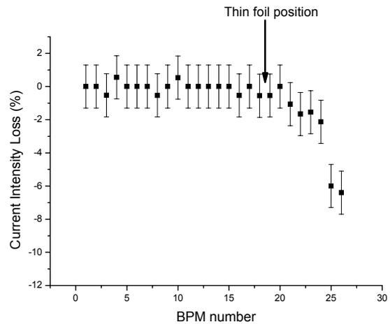
Figure 4: Current intensity loss in percentage as a function of the BPM number.
