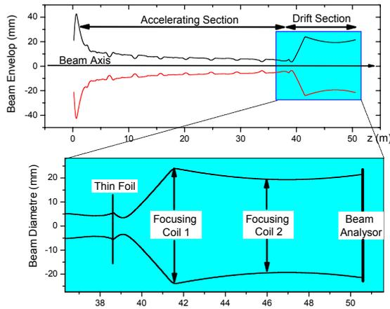
Figure 1: Expected e-beam envelopes into the both accelerating and drifting sections from TRAJENV. Reported positions correspond to the experimental arrangement.
