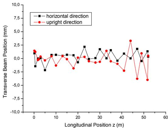
Figure 2: Beam centre motion from the diode to the X-ray converter.
