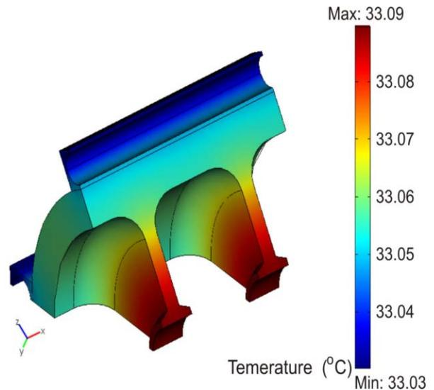
Figure 2: Accelerator structure 3D thermal model.
