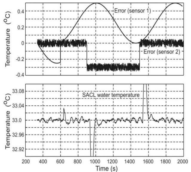
Figure 3: SACL water temperature stability simulation
