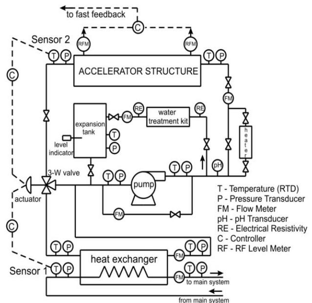
Figure 1: SACL water cooling system.
