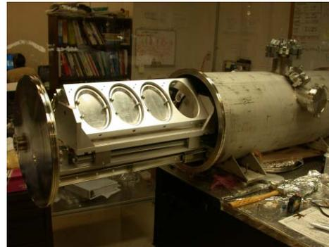
Figure 7: Optical Cavity Turning Mirror Cassette.
