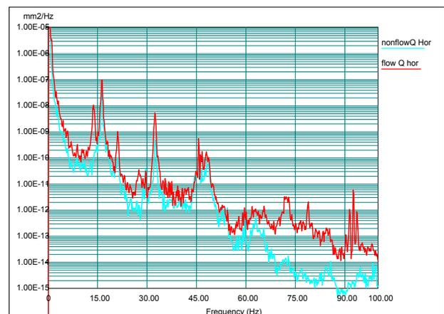
Figure 3. Compare the water flow and no flow on the Q magnet vibration in the horizontal direction.
