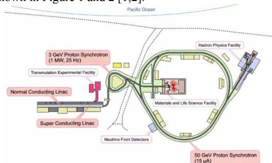
Figure 1: Layout of accelerators of the J-PARC [1].
