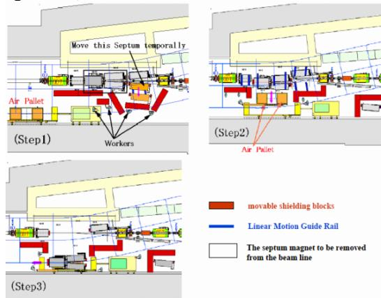
Figure 5: Carryout procedure for the septum magnet, the heaviest in the fast extraction system.
