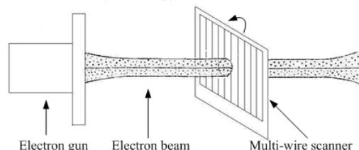
Figure 1: Beam profile measurement with rotating multi-wire scanner.
