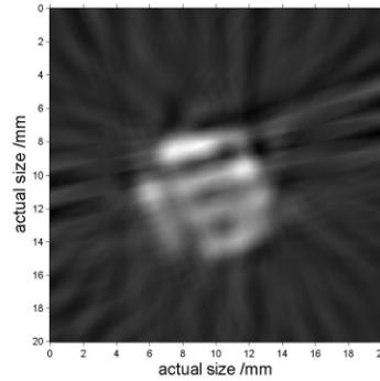
Figure 6: Beam profile reconstructed with mask (slit width 1mm).
