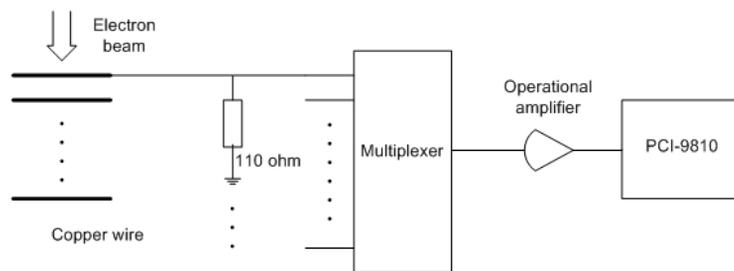
Figure 3: Schematic view of the wire signal measurement circuit.
