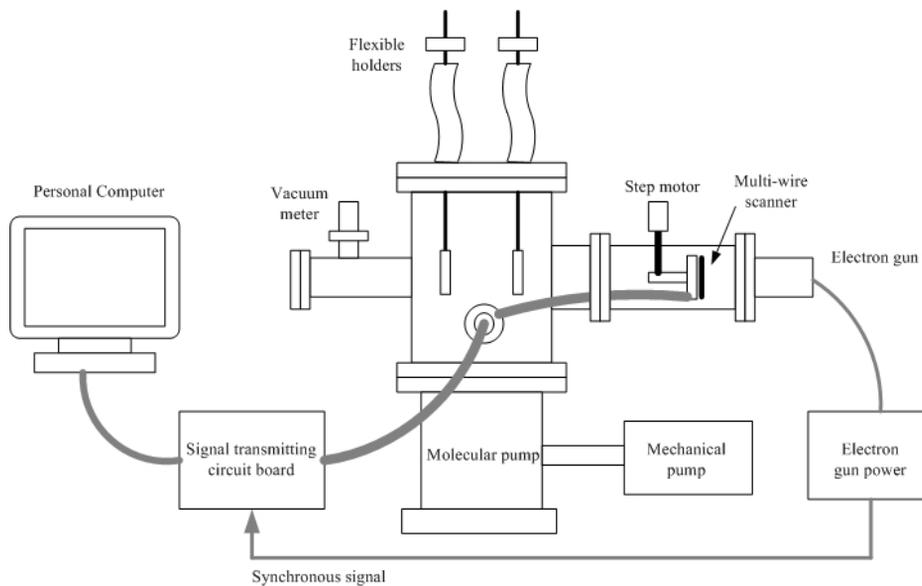
Figure 2: Schematic view of the experimental setup.
