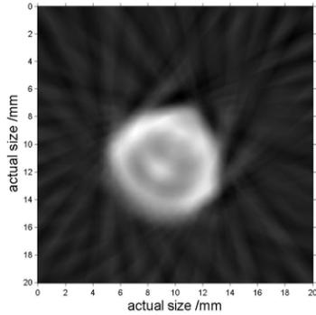
Figure 4: 2-D beam profile reconstructed.
