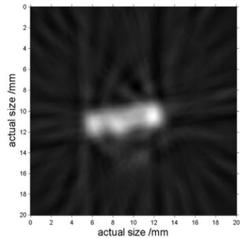
Figure 5: Beam profile reconstructed with mask (slit width 2mm).
