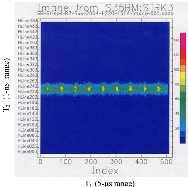
Figure 4: Dual-sweep streak camera image of the 324-singlets fill using the same ranges as Fig. 2. In this case the singlets are only four buckets apart and their spatial extent merges them into a horizontal band of light. The bunch length is 25 ps.
