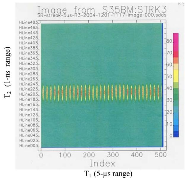
Figure 2: Dual-sweep streak camera image of the 24-singlets fill using a 1-ns vertical range (R3) and a 5- $\mu$ s horizontal range. All 24 singlets are seen individually in one turn plus a portion of a second turn. The bunch length is 40 ps.
