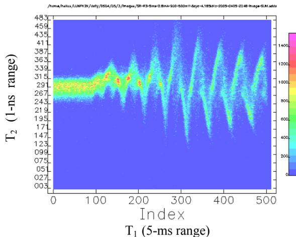
Figure 5: Dual-sweep streak camera image of a singlet fill with only 3 mA using a 1-ns vertical range and a 5-ms horizontal range. In this case the rf phase modulation technique results in a bunch length oscillation with compression of the nominal 35-ps bunch to 18 ps during the minimum of the oscillation.
