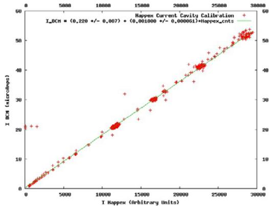
Figure 7: Calibration of the I cavity against the existing BCM cavity.
