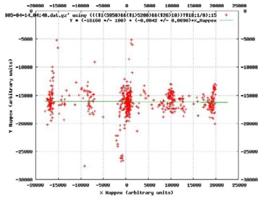
Figure 8: The X position was varied by  $\pm 2$ mm and no change observed on the Y position.
