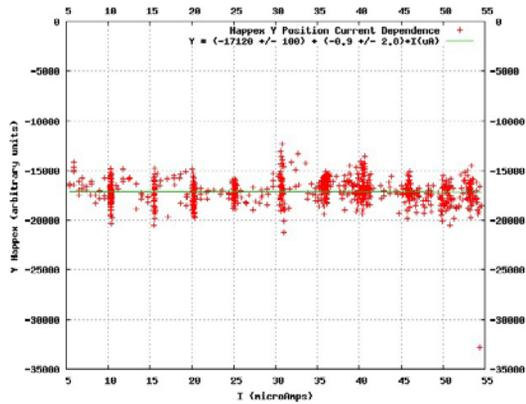
Figure 6: The Y position stayed constant as the current was changed from 1uA to 55uA.
