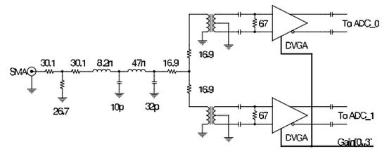
Figure 5: BPM front-end layout.
