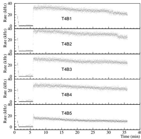
Figure 3: FLM bunch luminosity data for all bunches in a single train (Train 4).
