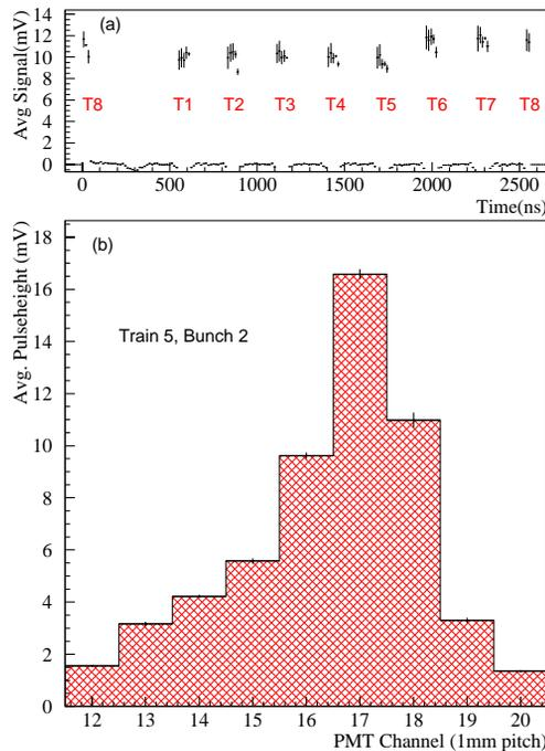
Figure 4: BSM prototyping data: (a) Timing scan showing the CESR  $e^-$  bunch structure during synchrotron light source operations (9400 turns per point); (b) Beam profile data obtained for a single  $e^-$  bunch for 500 turns as observed on the central PMT channels. The vertical scale for each plot is in units of the voltage produced at the PMT output termination.
