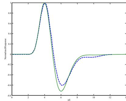
Figure 6: BPM front-end signal response. A PSpice simulation is shown by the solid (green) line while the prototype front-end data is shown by the dashed (blue) line.
