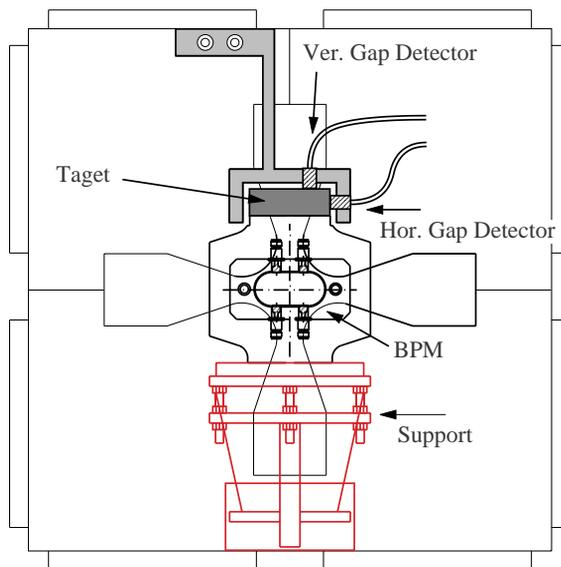
Figure 2: Gap detectors attached to QM
