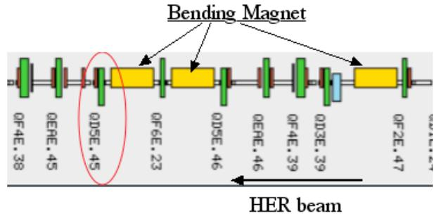
Figure 5: BPM located just downstream at the twin bending magnets.
