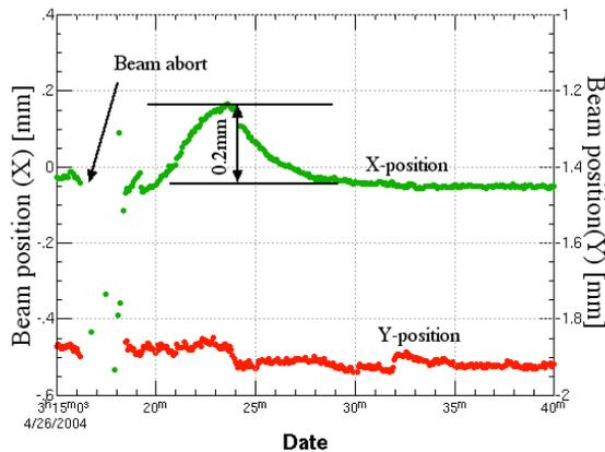
Figure 4: Change of BPM readings after a beam abort.
