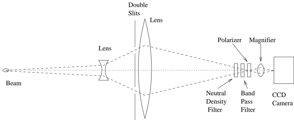
Figure 2: Retrofocus optics-equipped SR interferometer beam line.
