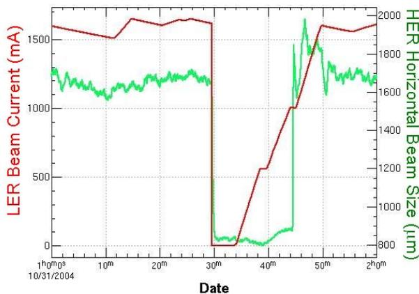
Figure 5: Measured HER horizontal beam size in collision and out of collision. The LER beam current (in red, left axis) is 1600 mA just before an LER abort at 1:30. The HER beam size (in green, right axis) is about  $1650\mu\text{m}$  in collision just before the abort, dropping to  $850\mu\text{m}$  out of collision, just after the abort.
