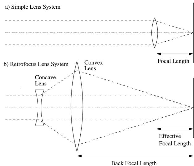
Figure 1: A) Simple lens system. B) Retrofocus (inverted telephoto) lens system with same effective focal length as a) but longer back focal length.
