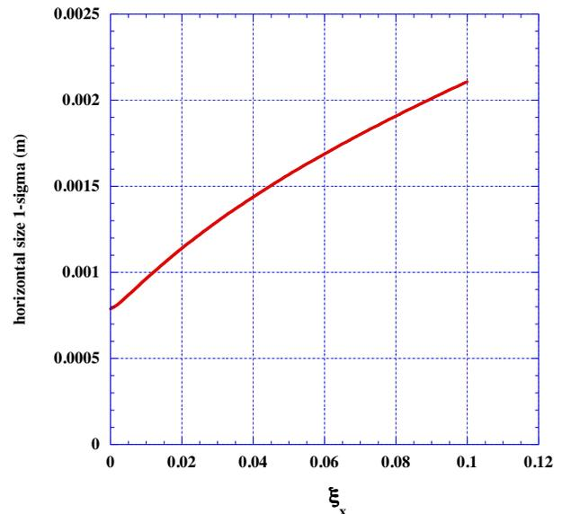
Figure 6: Calculated horizontal HER beam size at the SR monitor source point as a function of horizontal beam-beam parameter.
