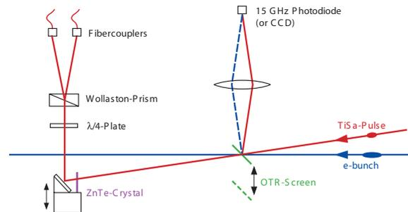
Figure 1: Schematic of the EOS setup. An OTR screen can be moved into the e-beam to adjust the relative timing between the laser pulses and the electron bunches with  $\approx 200$  ps precision.
