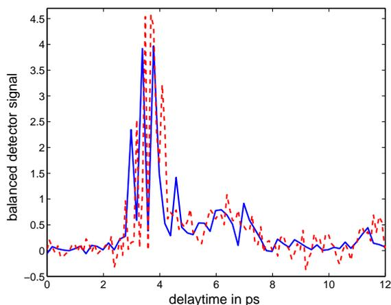
Figure 5: Two EOS measurements of short bunches, the second (dashed) measured approx. two minutes after the first (solid) (bunch charge 1.2 nC).
