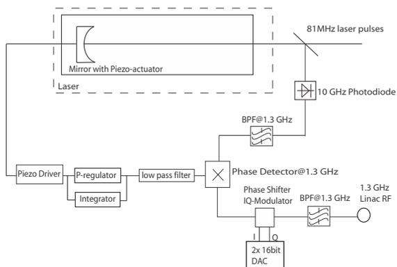
Figure 3: Schematics of the setup used to synchronize the laser to the RF. The laser repetition frequency is 81 MHz. The 16<sup>th</sup> harmonic of the laser frequency is phase-locked to the 1.3 GHz radio frequency of the linac.
