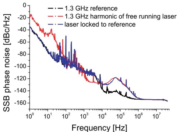
Figure 4: Phase noise of the 1.3 GHz reference signal, the free running laser and the laser locked to the reference.
