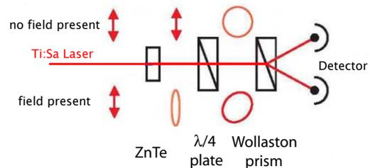
Figure 2: Simplified view of the signal detection using a quarter-wave plate, Wollaston prism and a balanced diode detector. The laser and the field of the bunch are polarized horizontally, parallel to the  $(-1,1,0)$  axis of the ZnTe crystal.
