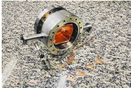
Figure 2: LNL XR BPM. It is possible to see the electrical feed-through, the blades and the isolating plates and tubes. The mask is mounted in a CF100 flange, the internal aperture for the beam is about 20 mm x 74 mm and the blades are about 25 mm decentralized. As shown in figures 1 and 2, the electrical connector can be installed in two positions, in order to facilitate the installation in different front ends.
