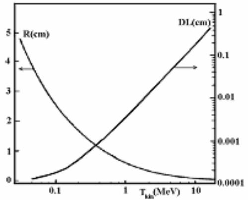
Figure 3: The dependence of  $R$  (left ordinates) and  $DL$  (right ordinates) on kinetic energy of the beam  $T_{kin}$ .
