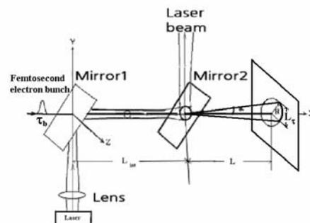
Figure 1: The scheme of the laser oscilloscope.
