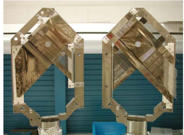
Figure 1: Shown at left (right) is a SEM paddle with strips at 0.5mm (1.0mm) pitch. Each wider exterior foils for measuring beam halo. The outer bias foils have been removed for clarity, but the middle bias foil is visible.
