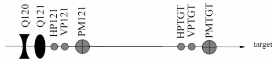
Figure 3: Schematic of the beam instrumentation upstream of the NuMI target, including two horizontal and two vertical BPM's, as well as two profile monitors.
