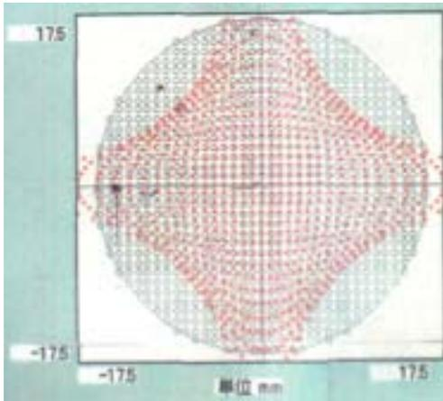
Figure 2: Simple reconstruction of position during online data taking. Red points for reconstructed position, and black points for wire position. This is for BPM with 37.7 mm diameter and scan is done by 1 mm step.
