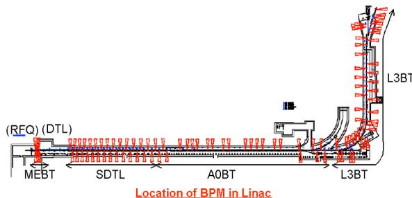
Figure 1: Location of BPM in the J-PARC LINAC. (LINAC consists of, from upstream, IS, LEBT (not shown), RFQ, MEBT, DTLs, SDTLs, A0BT, and L3BT (then connected to RCS synchrotron).) The tips of red arrows are the locations on the beam line.
