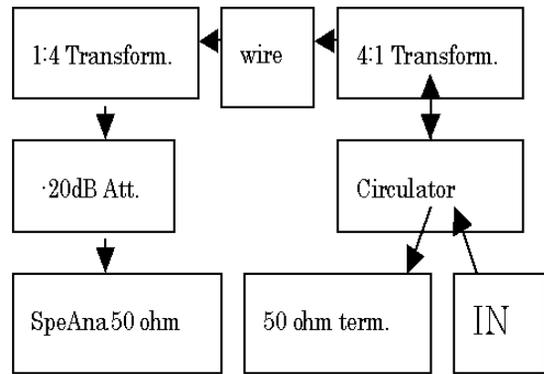
Figure 3: Configuration around scanning wire for calibration at test bench. Signal generator (324 MHz) is shown as "IN" in this diagram.
