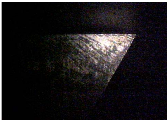
Figure 2: Side view of Tungsten slit with a 30° taper.
