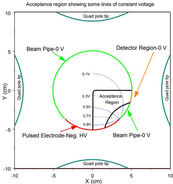
Figure 5: Acceptance limits of the nominal configuration.
