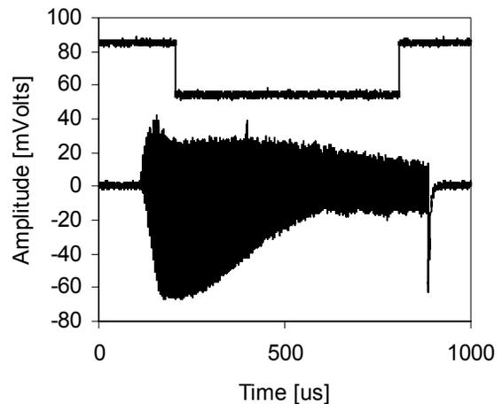
Figure 3: Wall current monitor signal with hardware gate.
