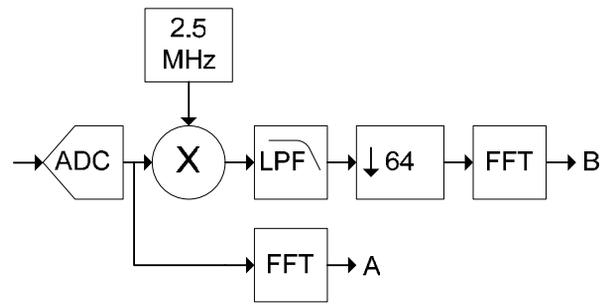
Figure 6: Signal processing chain.
