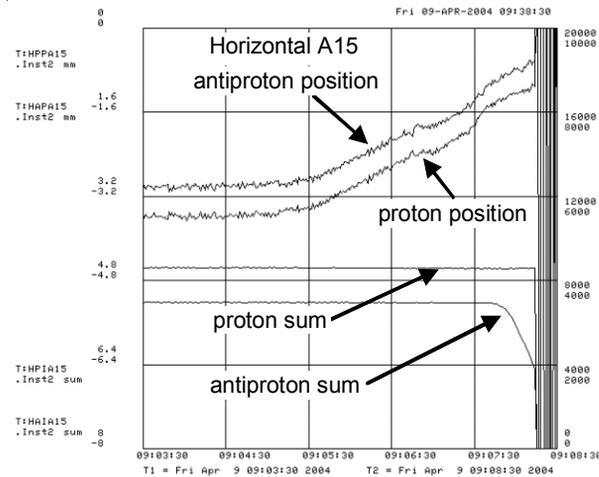
Figure 4. Horizontal proton and antiproton position (one scale inverted) and sum measurements during separator scan. Vertical: 1.6 mm beam position per division. Horizontal: 60 seconds per division.
