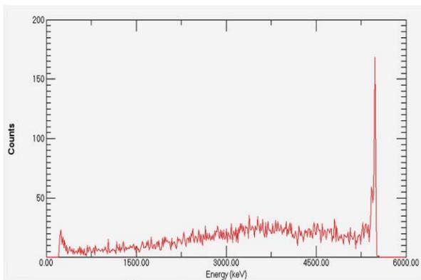
Figure 7: Energy spectrum of  $^{241}\text{Am}$   $\alpha$  particle using a 5-mm-thick Si surface barrier detector. A typical detected flux corresponds to  $2.23 \text{ mm}^{-2}\text{s}^{-1}$  and the 5.486 MeV main peak is visible.
