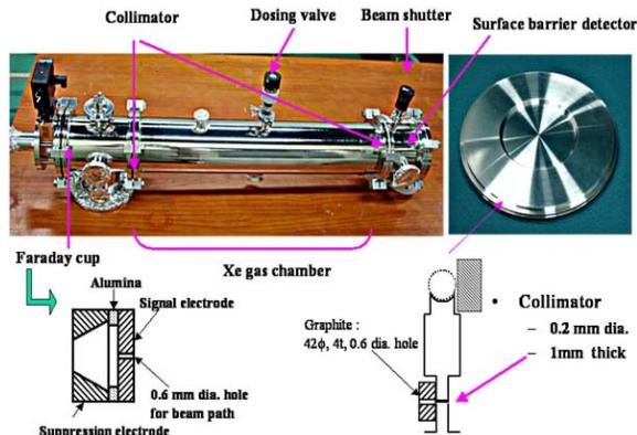
Figure 4: Photograph of gas scattering energy monitor with a faraday cup.
