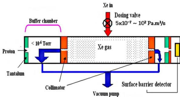
Figure 2: Structure of gas scattering monitor with a detector, two collimators, and a Xe gas chamber.
