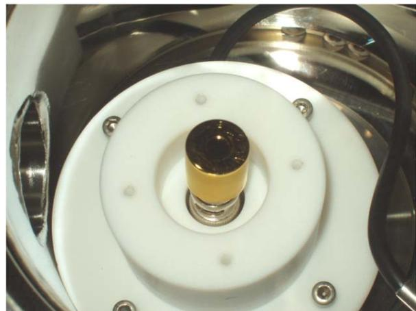
Figure 1: Photograph of the surface barrier detector installed in the gas scattering chamber.
