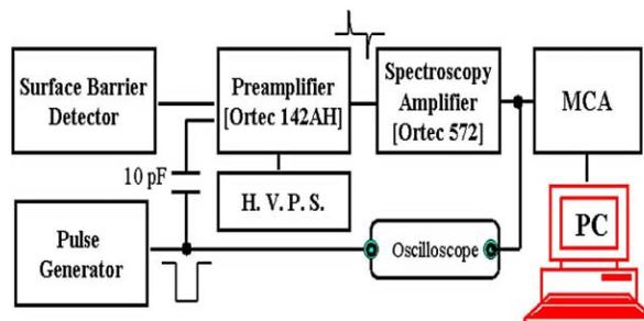
Figure 5: Schematic diagram of signal processing for energy measurement and energy calibration.
