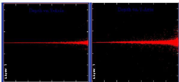
Figure 3: Gas scattering calculation by SRIM code: left for 10 Torr Xe, and right for 100 Torr Xe.
