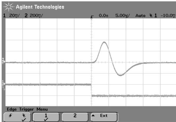
Figure 6: Input pulse and output signals from the pulse generator and the spectroscopy amplifier.
