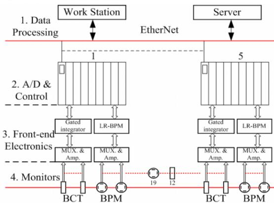
Figure 2: Block diagram of the DAQ structure.
