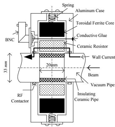
Figure 1: Schematic drawing of the BCT monitor.
