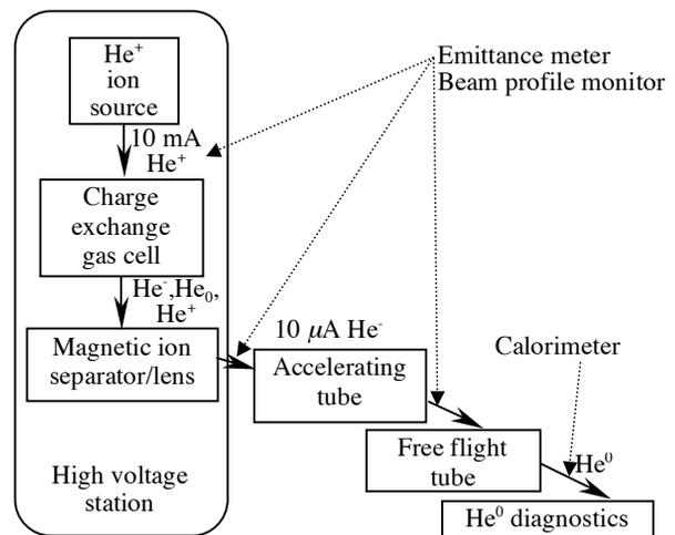
Fig. 2. Schematic diagram of the fast neutral He beam system under construction.
