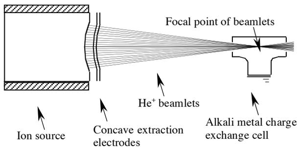
Fig. 1. Concept of converging  $\text{He}^+$  beam injection into a double charge exchange cell.
