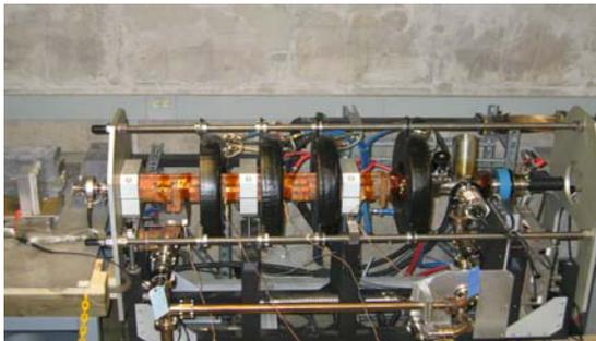
Figure 1: Accelerator system electron gun is on the right and beam exit is on the left.
