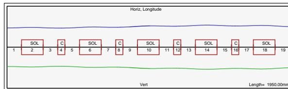
Figure 4: 500 mA 20 MeV Ne<sup>1+</sup> Beam in 15 T, 15 cm solenoid lattice separated by 25 cm including accelerating cavities.
