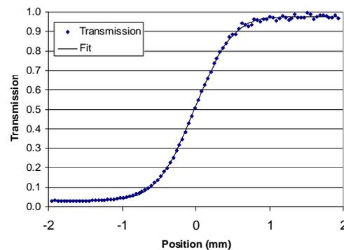
Figure 5: Electron radiograph collected from a prototype system (top). The edge transition as measured from the above radiograph and a fit of the transition expected from a Gaussian line spread function with an RMS width of 350  $\mu\text{m}$  (bottom)
