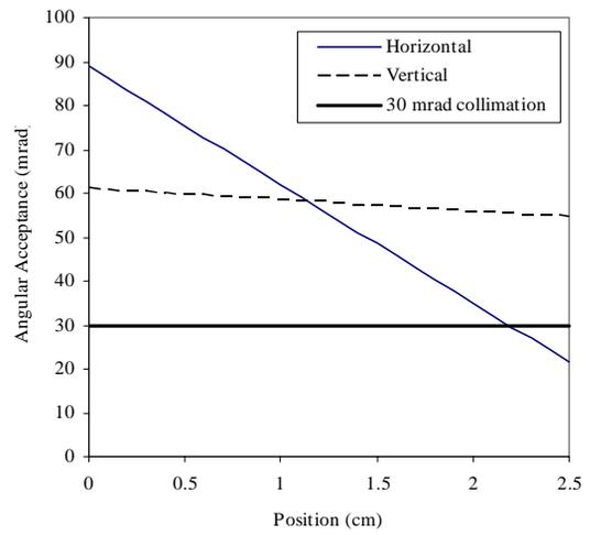
Figure 3: Horizontal and vertical angular acceptance as a function horizontal and vertical offset (respectively) from CPR lens axis.
