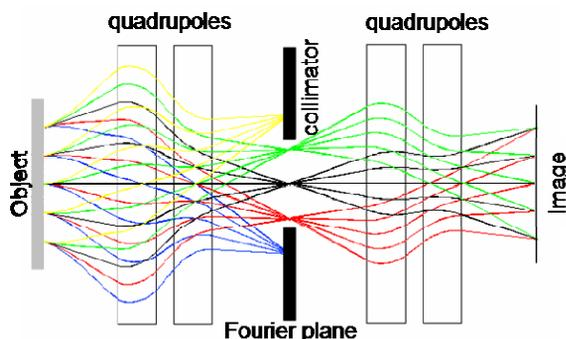
Figure 1: Schematic diagram of a CPR beam-optics system showing the point-to-point focus of particle trajectories (colored lines) from object to image. The colors represent the magnitude of scattering within the object. The Fourier point is located at the midpoint of the lens, where a collimator is positioned. The position-angle correlation at injection determines the location of the Fourier plane as well as partially cancelling second order chromatic aberrations.
