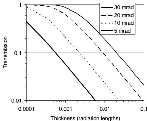
Figure 4: Transmission versus thickness in units of radiation length with a 5, 10, 20 and 30 mrad collimator.
