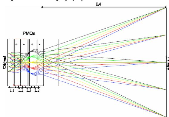
Figure 2: Schematic diagram of the CPR lens design described here showing the x5.9 magnification point-to-point focus of particle trajectories (colored lines) from object to image.
