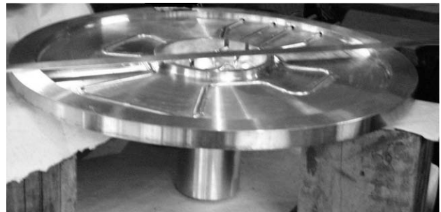
Figure 2: Disk of accelerating structure during manufacturing.
