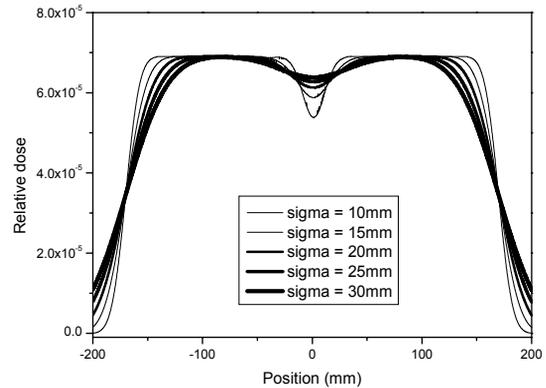
Figure 3: Dose distribution with various beam sizes.
