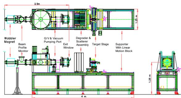
Figure 1: 50MeV beamline which is attached to the MC-50 cyclotron at KIRAM.
