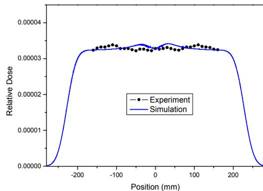
Figure 4: A fluence distribution measure by film dosimeter and calculation result of spiralscanning method
