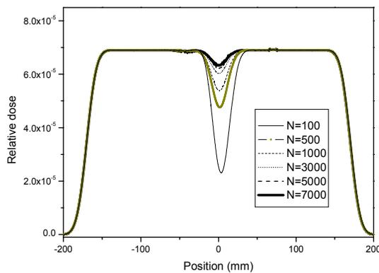
Figure 2: Number of revolutions vs. relative dose ( $\sigma = 10mm$ ,  $R = 170mm$ ).
