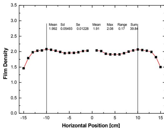
Figure 6: A fluence distribution measure by film dosimeter of mechanical wobbler method.
