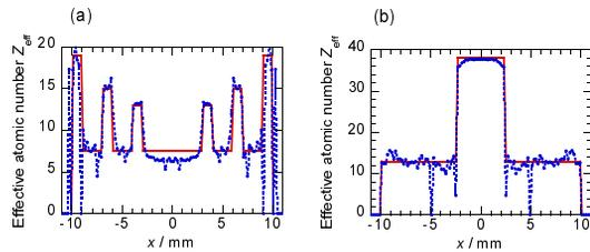
Figure 5: Atomic number distributions at  $y = 0$  for sample and reconstructed images in (a) Fig. 4 and (b) Fig. 6. The dotted line indicates effective atomic number  $Z_{\text{eff}}$  and the solid line indicates atomic number of the sample.
