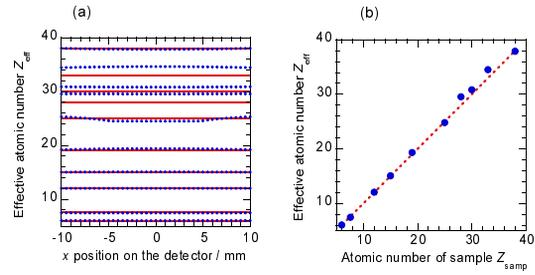
Figure 3: (a) Effective atomic number  $Z_{\text{eff}}$  on each pixel of the detector. The solid circles indicate identified effective atomic number  $Z_{\text{eff}}$ . (b) Average of the effective atomic numbers.
