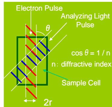
Fig.2 Concept of equivalent velocity spectroscopy
