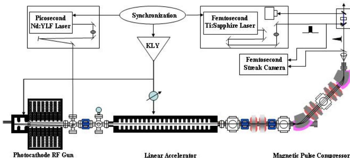
Figure 1: Block diagram of femtosecond pulse radiolysis system.
