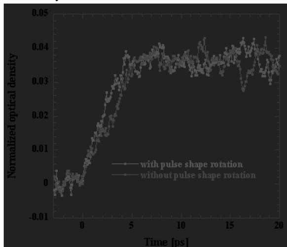
Fig. 3, optical absorption of hydrated electron in water measured with equivalent velocity spectroscopy at 800nm.
