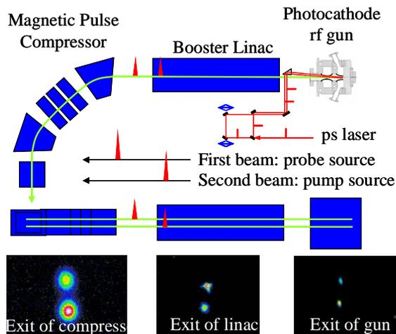
Fig. 4 A double-decker electron beam generation system.
