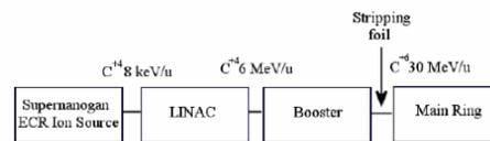
Figure 1: The base injection scheme.
