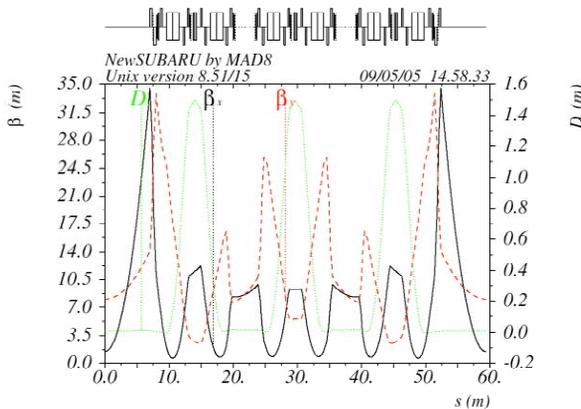
Figure 1; Lattice functions (the half of the ring) in the quasi-isochronous (low  $\alpha$ ) mode calculated by MAD.
