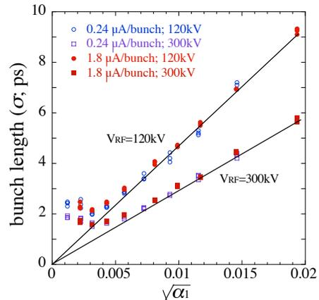
Figure 2; Momentum compaction factor  $\alpha$  vs. RMS bunch length measured by a streak camera.
