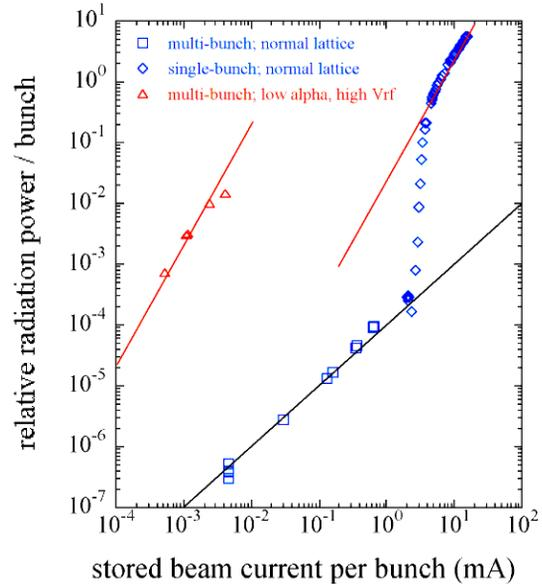
Figure 4; CSR power vs. stored current per bunch. (square: normal  $\alpha$  with multi-bunch, diamond: normal  $\alpha$  with single bunch, triangle: low  $\alpha$  with multi-bunch)
