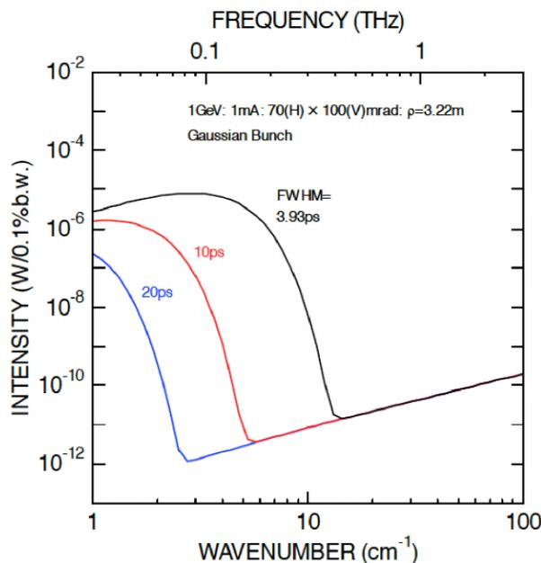
Figure 6; Calculated CSR power spectrum from the planning extraction port with larger aperture.
