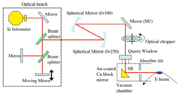
Figure 3; Setup of CSR spectrum measurement. In case of power measurement, CSR is directly feed from M1 mirror to Si bolometer.
