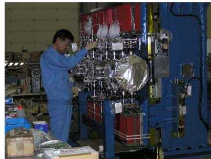
Figure 2: Picture of the first ALS in-vacuum undulator with 3 cm period and 1.52 T maximum field being assembled at Neomax.
