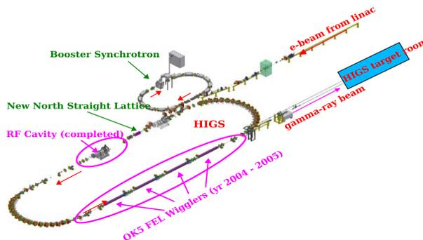
Figure 1: Fully upgraded Duke storage ring light source facility in 2006 with a HOM-damped RF cavity, a new 0.25 – 1.2 GeV booster, a new straight section for the OK-5 FEL, a second new straight section for booster injection and future light sources.
