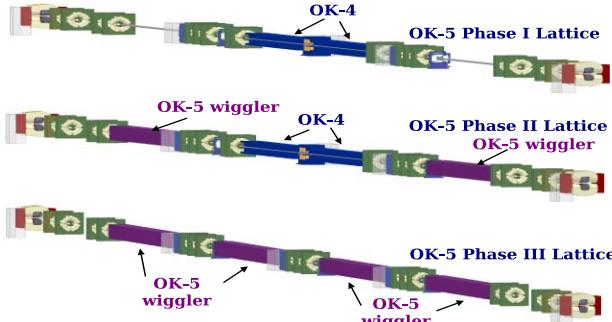
Figure 2: Three phases of the OK-5 FEL straight section lattice.
