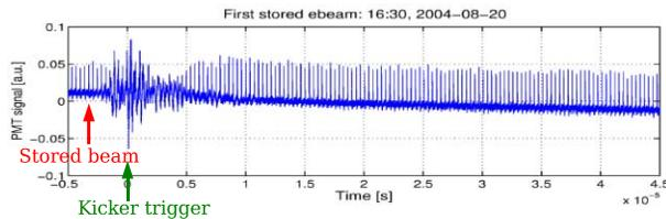
Figure 3: First stored beam captured by a photo-multiplier.
