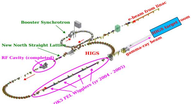
Figure 1: Fully upgraded Duke storage ring light source facility in 2006 with a HOM-damped RF cavity, a new 0.25 – 1.2 GeV booster, a new straight section for the OK-5 FEL, a second new straight section for booster injection and future light sources.
