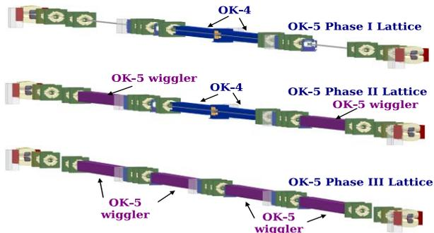
Figure 2: Three phases of the OK-5 FEL straight section lattice.
