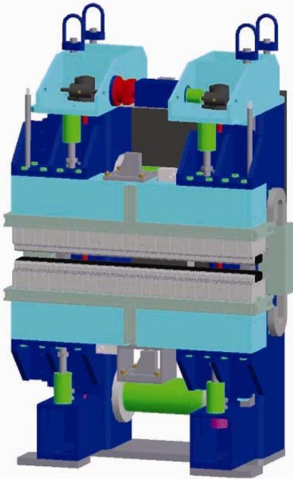
Figure 1: Draft version of the EUV undulator to be installed in a short straight section. Courtesy of ADC. [2]
