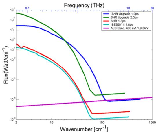
Figure 1: SHR CSR power spectrum horizontal acceptance/port: 300 mrad for upgrades, 60 mrad for all others.
