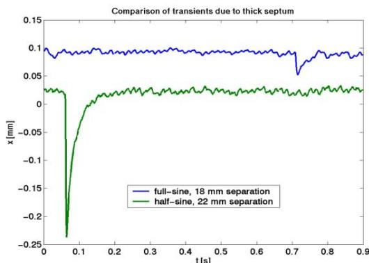
Figure 3: Transients for full (blue) and half (green) wave sinusoidal excitation. Note: \*\*Acquisition of data for two curves is not synchronized. Peaks are coincident with each other.
