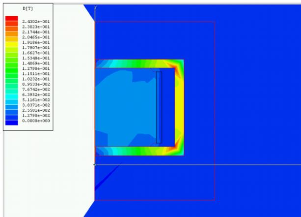
Figure 2: HFSS Half magnet simulation of B field @ 1.9 GeV.
