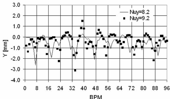
Figure 1: Vertical COD due to vertical correctors.
