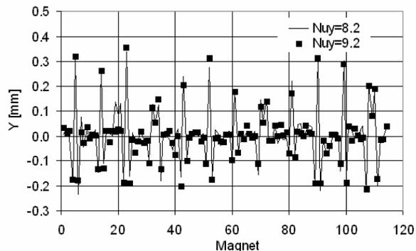
Figure 2: Effective vertical misalignments along the circumference.
