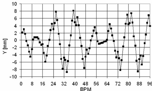
Figure 4: Uncorrected Vertical Orbit of LILA.
