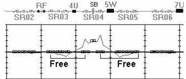
Figure 5: Parallel bump for superbend in sector 4 showing the area where BPMs are not used (marked as Free),  $N_{uy}=9.20$ , vertical full scale  $\pm 10$  mm.
