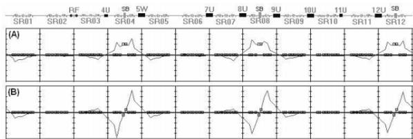
Figure 4: Parallel (A) and angle (B) bumps at 3 superbends,  $N_{uy} = 9.2$ , vertical full scale  $\pm 10$  mm.
