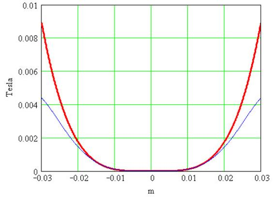
Figure 6: Decapole configuration  $\frac{\partial^4 B}{\partial x^4} = 2.64 \cdot 10^5 \cdot \frac{\text{Tesla}}{m^4}$
