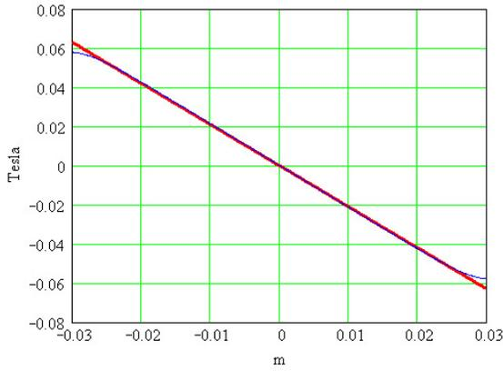
Figure 3: Quadrupole configuration  $\frac{\partial B}{\partial x} = -2.1 \cdot \frac{\text{Tesla}}{m}$
