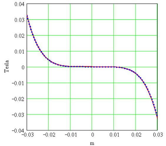
Figure 7: Dodecapole configuration  $\frac{\partial^5 B}{\partial x^5} = 1.62 \cdot 10^8 \cdot \frac{\text{Tesla}}{m^5}$
