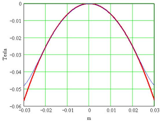
Figure 4: Sextupole configuration  $\frac{\partial^2 B}{\partial x^2} = 126 \cdot \frac{\text{Tesla}}{m^2}$
