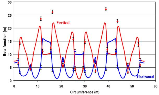
Figure 3: Measured and predicted beta functions for the new low emittance optic, including the 7 T wiggler.
