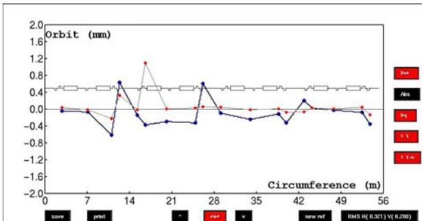
Figure 6: Corrected orbit referenced to the quadrupole centers for the low emittance optic. The horizontal (blue) rms is 0.32 mm, the vertical (red) rms is 0.28 mm.
