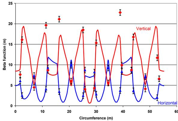
Figure 2: Measured beta functions for the small beta optic with the wiggler at 7 T. The wiggler location is at the center of the diagram.
