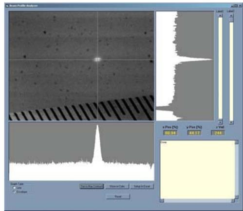
Figure 4: X-ray pinhole image with small beta optic and wiggler at 7 T.
