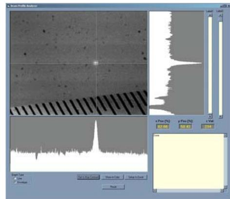
Figure 5: X-ray pinhole image with new optic and wiggler at 7 T.
