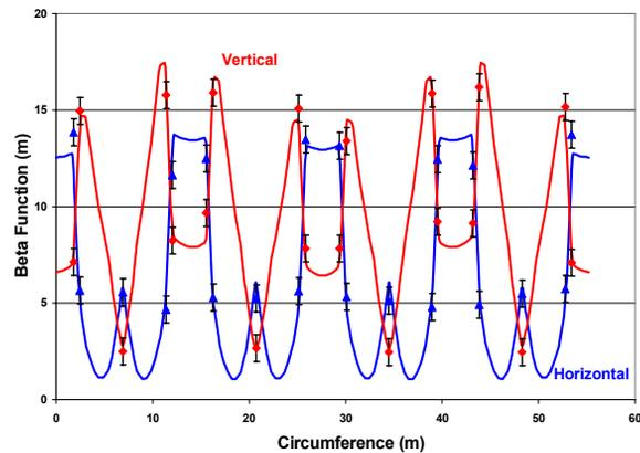
Figure 1: Measured beta functions, shown by the data points, for the basic lattice in its fully symmetric mode with the wiggler off. The solid lines are computed from the lattice model.
