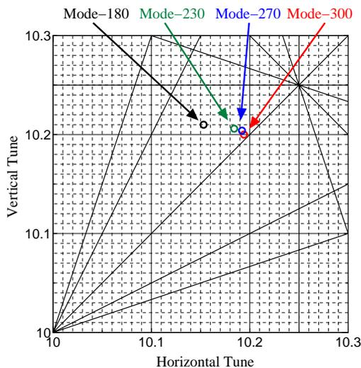
Figure 1: Tune diagram near the coupling resonance. For the medical application, we can change the operating point to following 4 modes, Mode-180, Mode-230, Mode-270, and Mode-300. These modes correspond to the vertical beam size.
