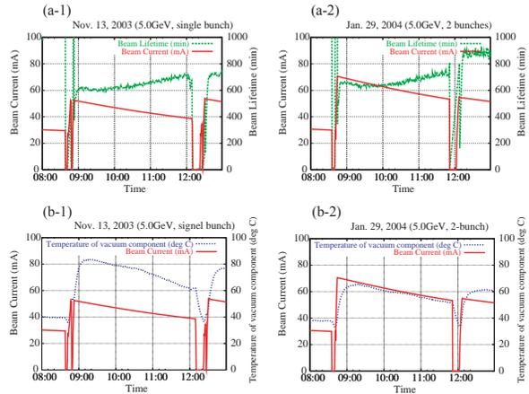
Figure 2: The beam current and the beam lifetime during the medical application for (a-1) single bunch and (a-2) 2-bunch operation. And the beam current and the temperature of the vacuum components adjacent to an RF cavity for (b-1) single bunch and (b-2) 2-bunch operation.
