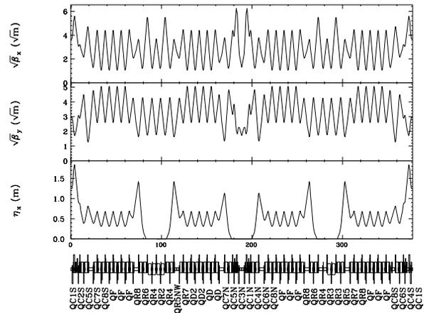
Figure 3: Optical functions in the PF-AR under the medium emittance optics.
