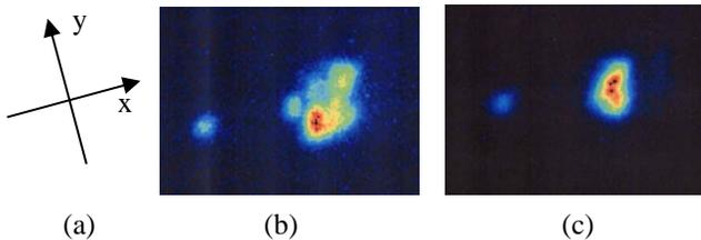
Figure 2: Result of coherent oscillation of the beam before an optimization of pulse bump (b), and after an optimization of pulse bump (c). Coordinate system in these figures is rotated 12° in CCW manner due to alignment of optical system as indicated in (a).
