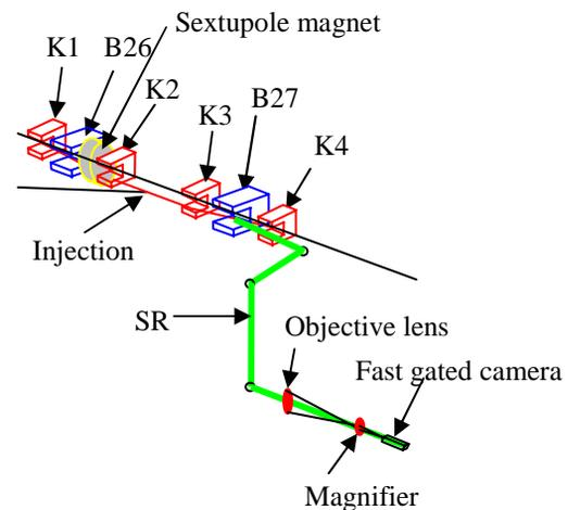
Figure 1: Arrangement of kicker magnets and optical layout of the SR monitor. K1,2,3,4 denote kicker magnet No.1,2,3,4, respectively. B26,27 denotes bending magnet No.26, and 27. The quadrupole magnets are omitted in this figure.
