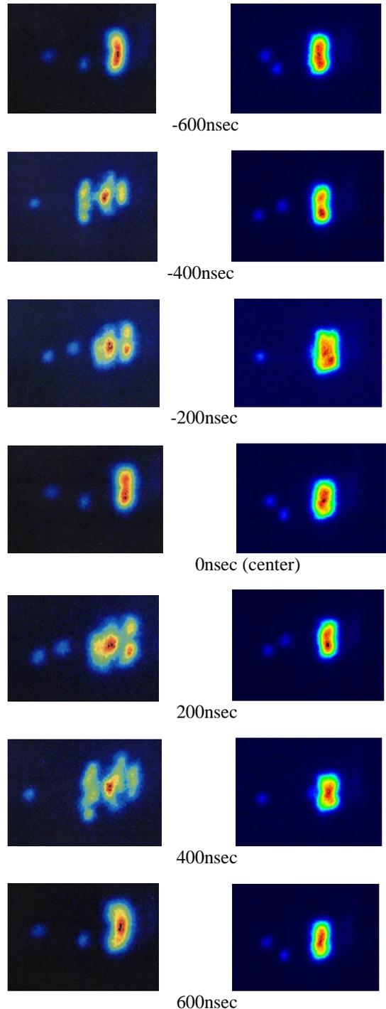
Figure 4: The results of observations of the stored beam oscillation with (left column) and without (right column) the sextupole magnet.
