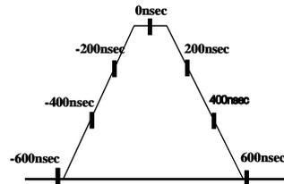
Figure 3: The relation between measuring points of timing and pulse shape of the injection bump.
