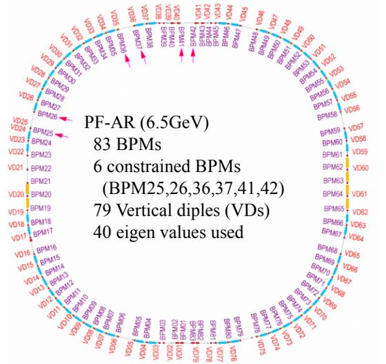
Figure 1: Configuration of the BPM and vertical orbit correction system at the PF-AR.
