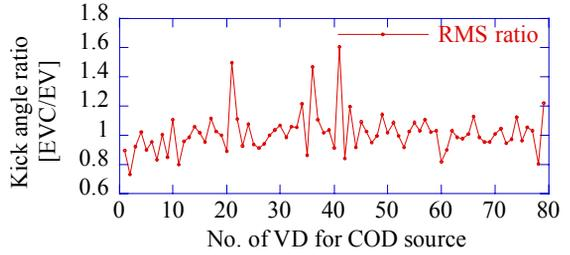
Figure 5: RMS ratio of the kick angles of the steering magnets.
