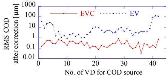
Figure 7: RMS of the COD at the constraint point for the PF ring.
