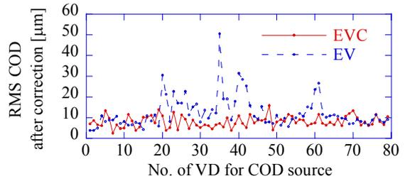
Figure 3: RMS of the COD at the constraint point for the PF-AR.
