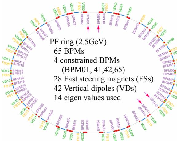
Figure 2: Configuration of the BPM and vertical orbit correction system at the PF ring.
