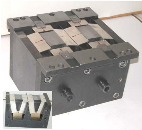
Figure 5: Lower half of the short prototype wiggler.
