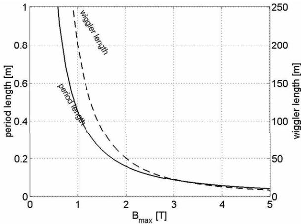
Figure 2: Maximum period length (solid) and required wiggler length (dashed) for a given peak field of a sinusoidal wiggler.
