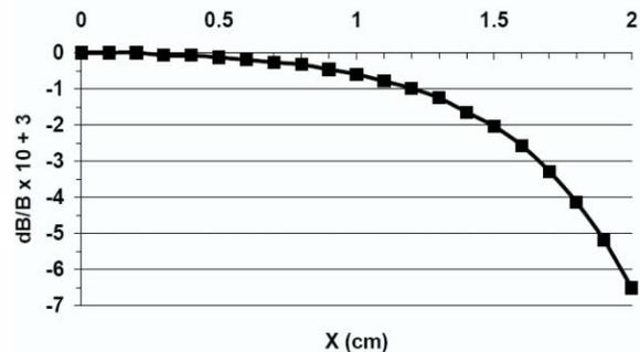
Figure 4: Transverse magnetic field distribution.
