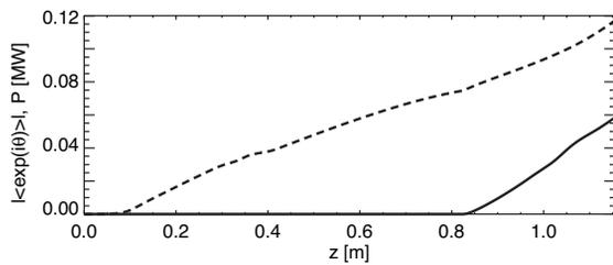
Figure 2: Growth of the radiation power and current modulation (solid and dashed line, respectively) at  $102 \mu\text{m}$  along the Neptune beam line. The waist position of the LBW is positioned at  $z = 9 \text{ cm}$ .
