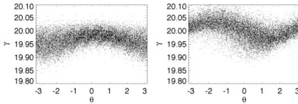
Figure 3: Longitudinal phase space distribution ( $\theta = (2\pi c/\lambda)t, \gamma$ ) at the waist position of the LBW and at the exit of the undulator (left and right plot, respectively) for  $\lambda=102 \mu\text{m}$ .
