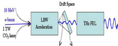
Figure 1: Conceptual design for the Neptune experiment.
